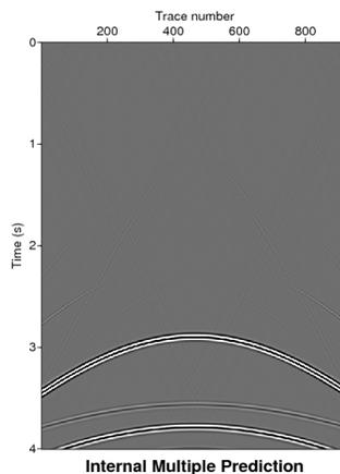
Figure 4: Prediction of all the first-order internal multiples.
